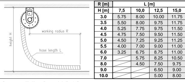
R Working radius rounded off to 0.25 m accuracy •••
